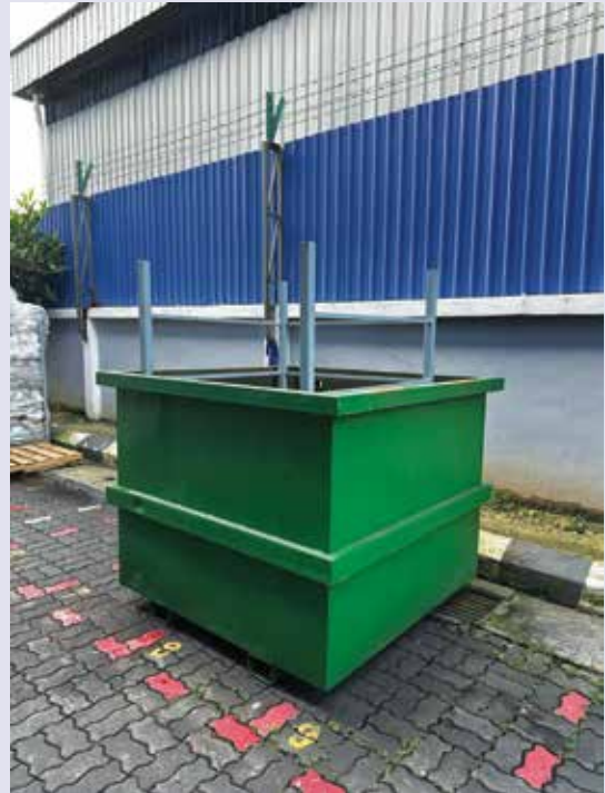
Water Tank for Leaks test
