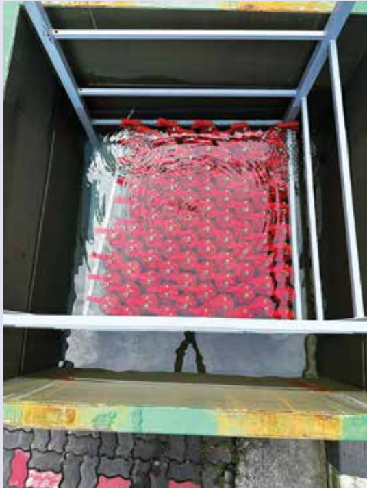
CO 2 Fire Extinguisher Leaks Test Process
